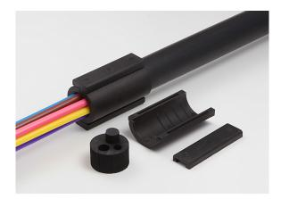
Suitable for gas and watertight sealing of 32mm HDPE ducts, which contain mini ducts and / or (fibre optic) cables. The modular system will guarantee easy installation of various different cable and duct configurations. Our system is divisible so can be applied at installation or afterwards. The rubber inserts can be custom designed for your specific needs and configuration and will contain (temporary) blind plugs to make the system more flexible at the installation site.
